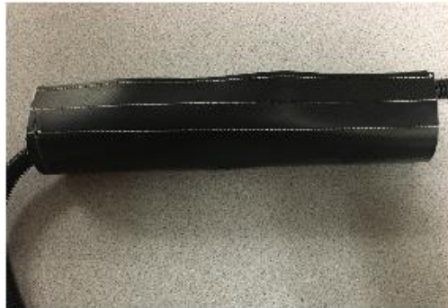
Step 2: Securely wrap the two ends of the protective sleeve together making sure velcro is sealed on the top side of the front jump start plug holder.
