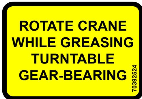
Crane worm gear bearing teeth must be lubricated weekly with lubriplate gear shield extra-heavy or equivalent, applied with a grease gun, caulk gun or brush. Cover all teeth with grease and leave no exposed metal surfaces showing.
