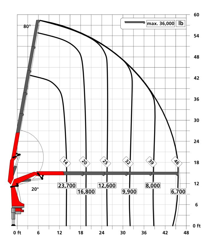
Symbolic crane figure, indications at 20° main boom position & load arm in horizontal position
